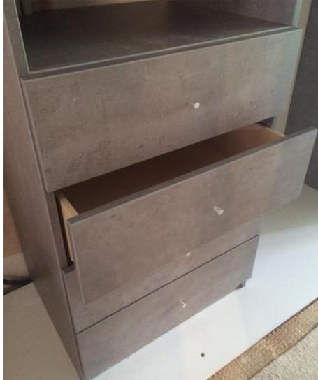
17. Finally fix handles. 370 and 150 series glass fronts, the aluminium frame can be drilled (5mm hole) anywhere 7mm in from the edge. 100 series 10mm in from the edge.
