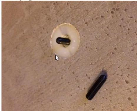
15. Screw into the adjusters and offer front to box. When happy with position push the front onto the box to give hole location marks. Drill using a 6mm drill bit. Use a block inside drawer to avoid break out.
