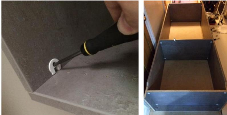
3. The multi drilled holes are at the top of the unit. Three fixed shelves hold the unit together. One at the bottom 5mm holes, a mid shelf first hole of the sequenced multi hole section (4 brackets are provided for additional support on the underside and the very top hole).
